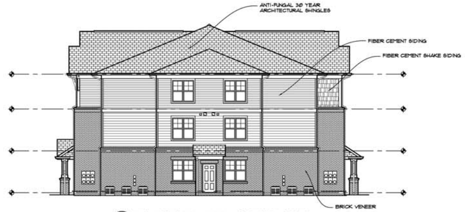
3 BUILDING 100 & 300 - SIDE ELEVATION 1/8" = 1'-0"
