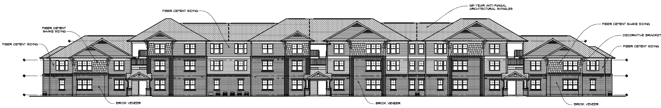
1 BUILDING 200 - FRONT ELEVATION (PARKING LOT) 3/32" = 1'-0"
