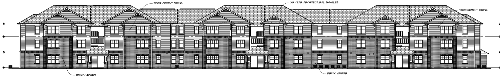
2 BUILDING 300 - REAR ELEVATION 1/16" = 1'-0"
