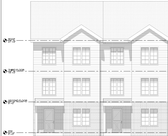
3 TYP. FRONT ENTRANCE ELEVATION (GARAGE UNIT) A201 1/4" = 1'-0"
