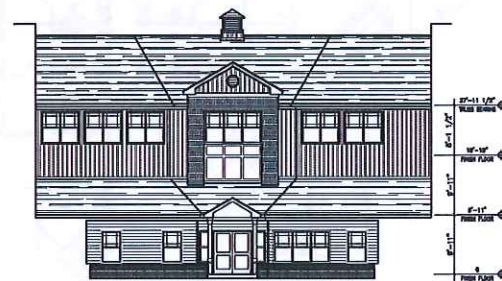
4 Partial Front Elevation - Core Area Scale: 3/32" = 1'-0"
