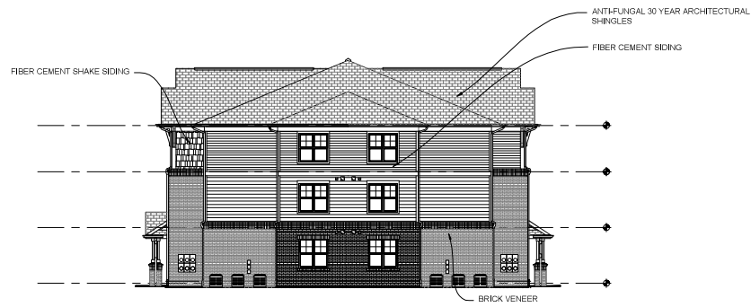
4 BUILDING 500 - SIDE ELEVATION 1/8" = 1'-0"
